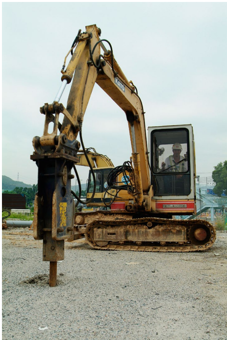
The use of power-driven grinding, chiselling, cutting or percussive tools on rocks
